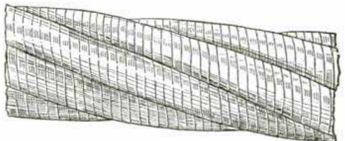
Wire Rope Covered with Flat Wire to Protect the Strands from Abrasion
