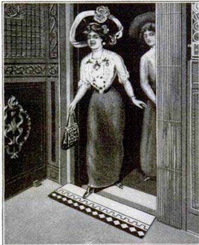
Yielding Section in Floor of Elevator Prevents Movement Up or Down When a Passenger is Standing Upon It
