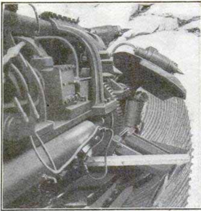
View of Head of Tunnel-Boring Machine and Sketch Showing Arrangement of the 15 Drills
