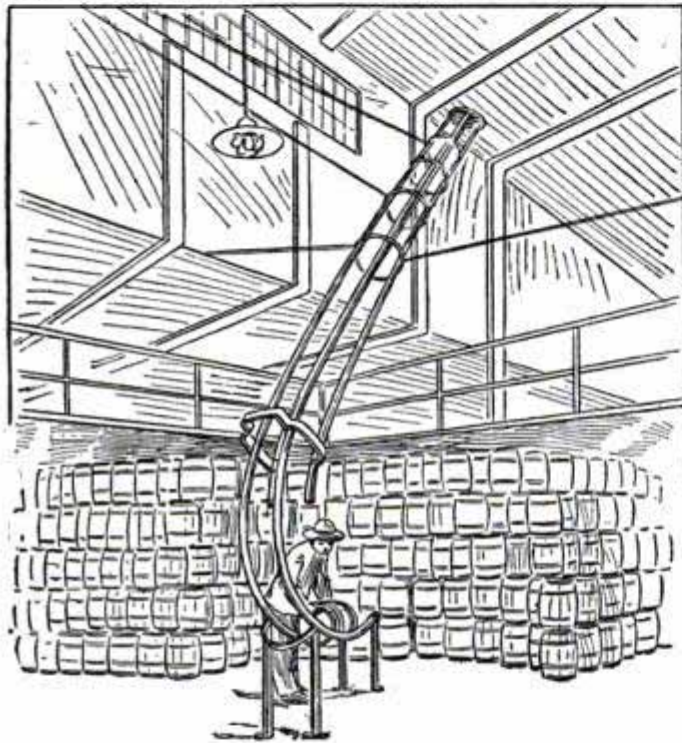
Gravity Chute at Delivery End of Keg Conveyor
