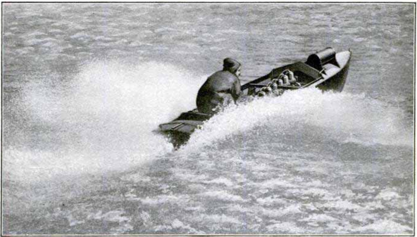
A Light Aeroplane Motor Pushing Motorboat through Water at Rate of 30 Miles an Hour
