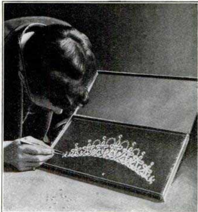
Making Up the Design of a Tiara in Wax. All the Stones are Placed in It, so That the Effect may be Viewed
