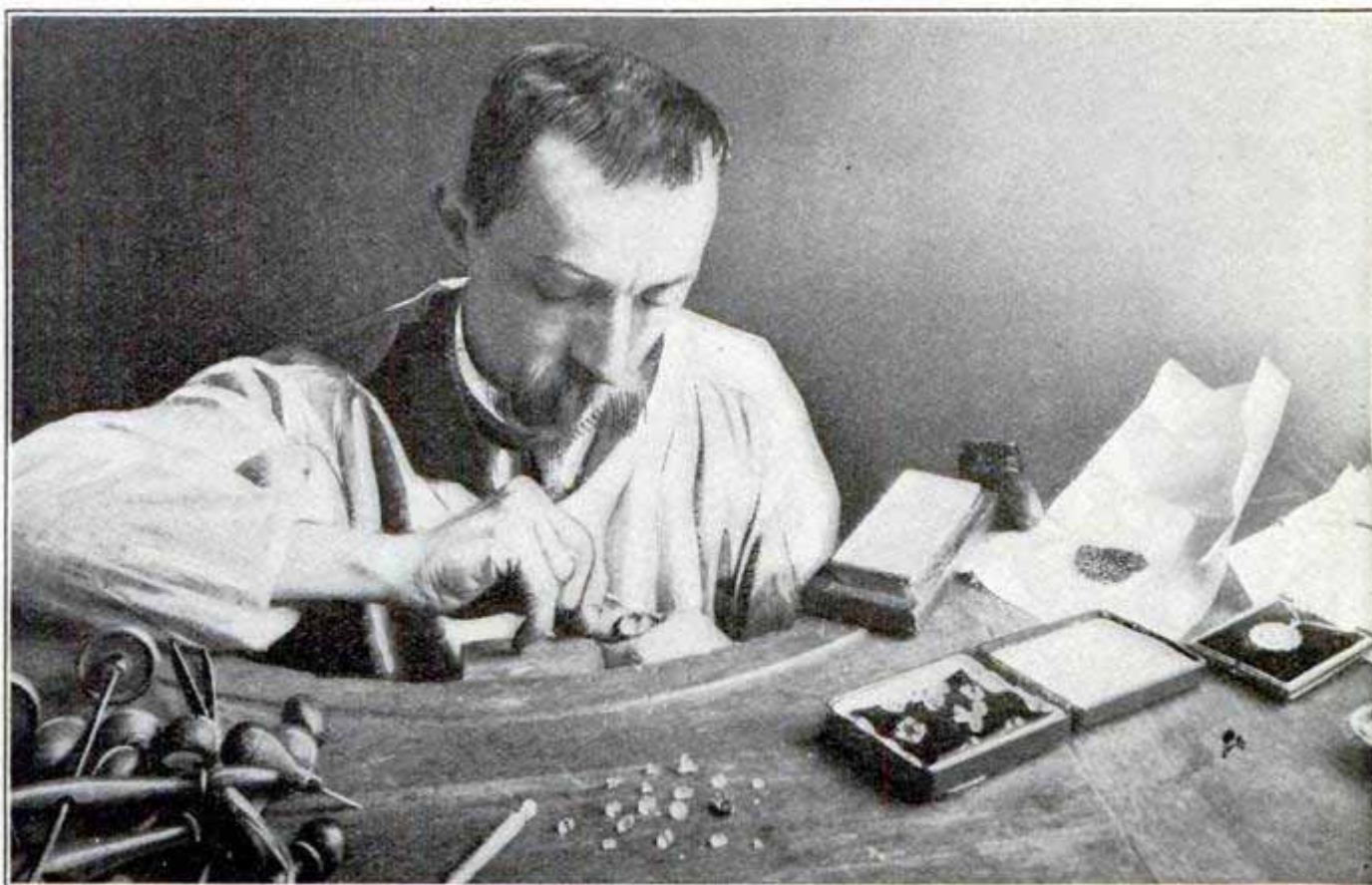
Setting One of the Large Stones in a Coronation Tiara. If a Single Workman were to Set All the Stones in a Good Tiara, It Would Take Him Seven Weeks to Complete One
