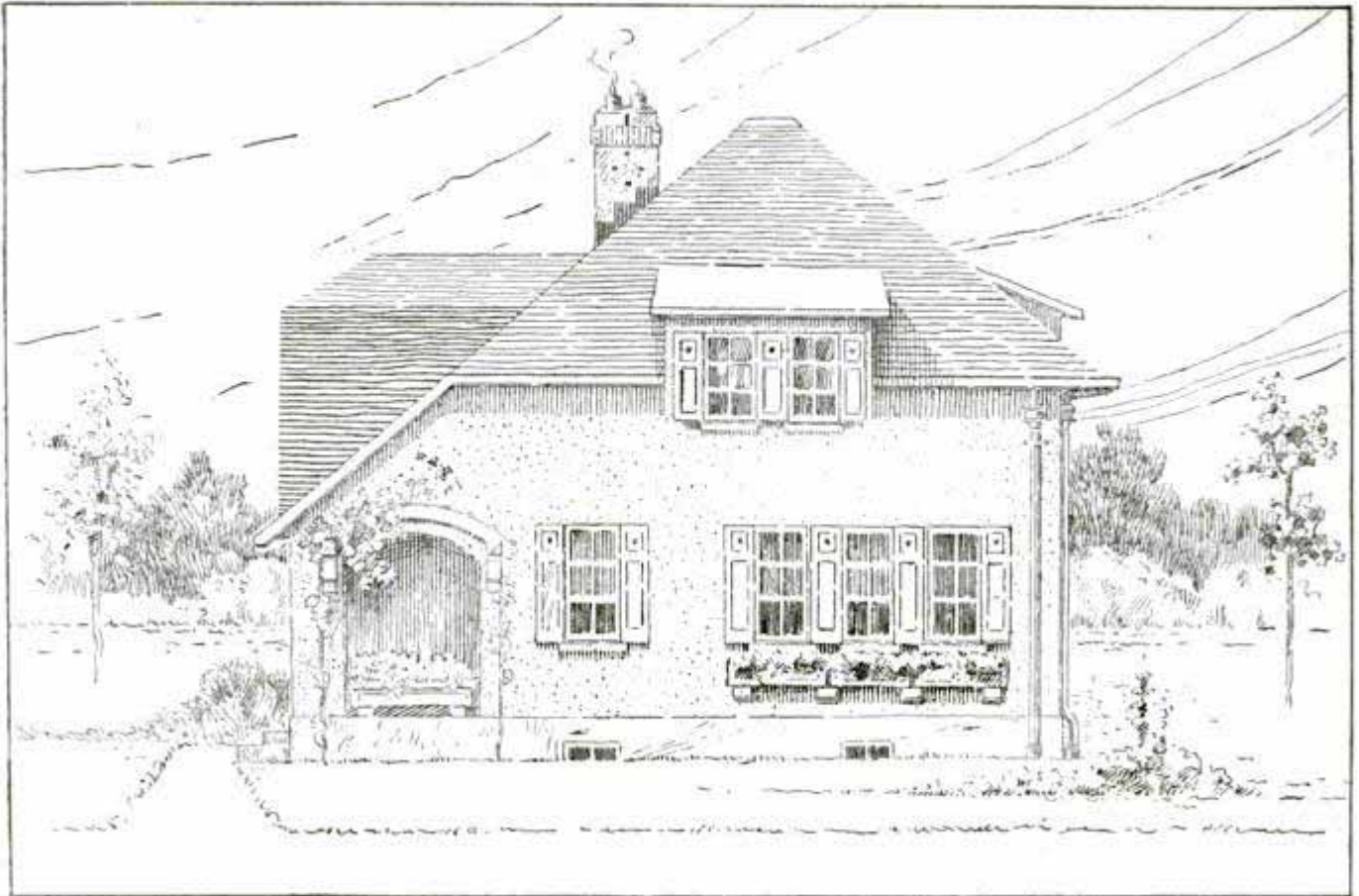
Front Elevation Showing Entrance Porch at the Side
