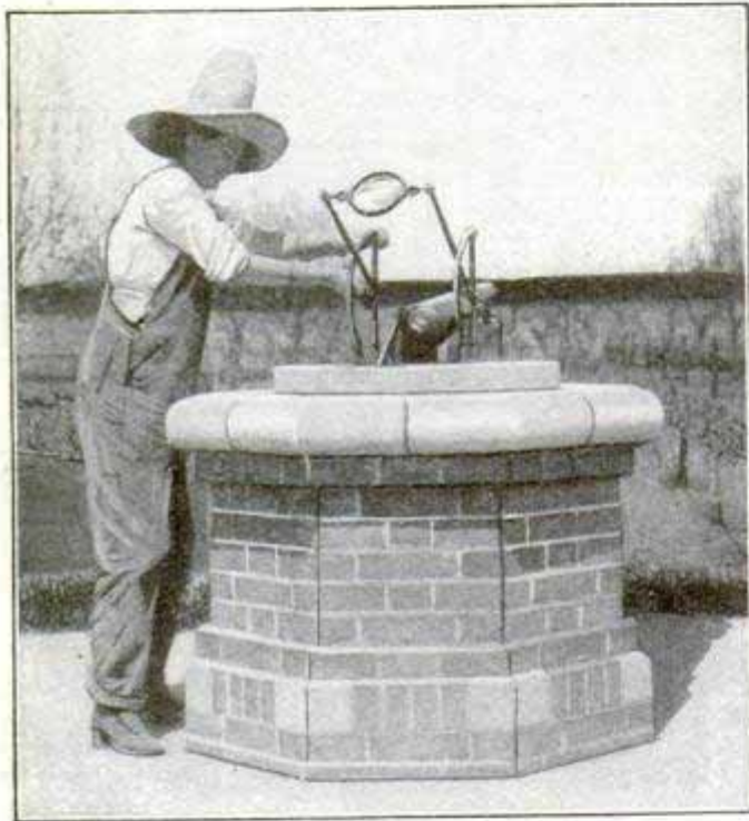
Adjusting the Sundial which Sets Off the Cannon Automatically at Noon
