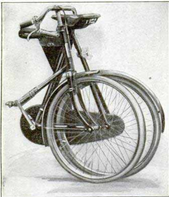
A Bicycle that Can be Folded Up and Carried in a Leather Case
