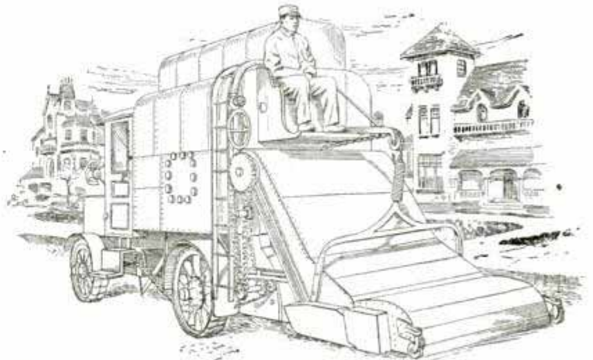
This Street-Cleaning Machine Sweeps Up the Debris, Conveys It into a Dust Compartment and Carries It to the Dump
