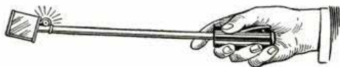
Portable Electric Lamp with Adjustable Mirror
