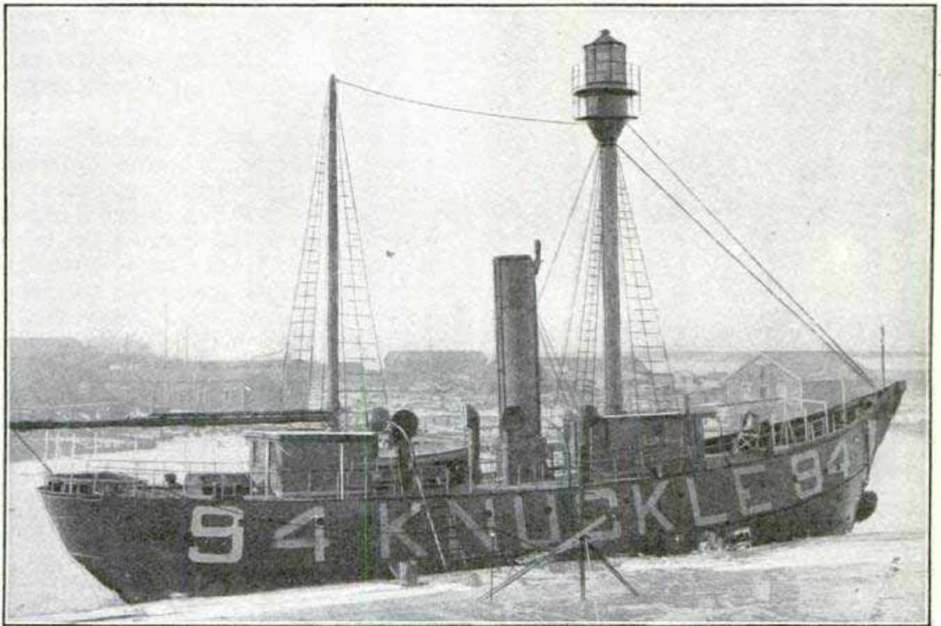
Equipped with a Revolving Light on a Hollow Mast Containing a Ladder, This is the Most Up-to-Date Light Ship in the Country
