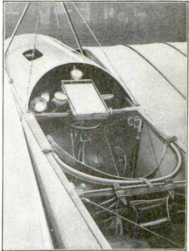
Pilot's Seat in New Bleriot Monoplane, Showing Maps, Compass, Watch, Barometer, and Revolution Indicator.
