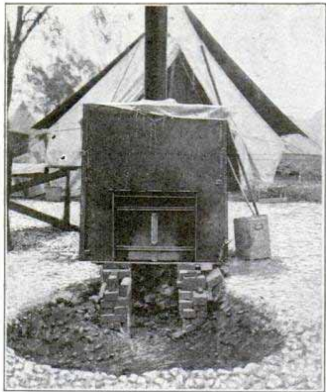
Rear View of Army Oven Showing the Fire Box
