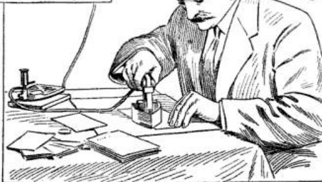
Mounting Prints by the Aid of an Electric Flatiron
