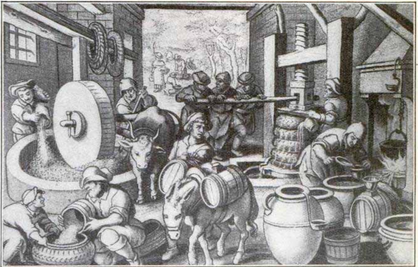
No. 6—AN OLIVE-OIL MILL.—The olive has been cultivated in Syria, Palestine, and other parts of the East since the earliest times. Its cultivation extends as far south as Cairo, and north to the middle of France. In the illustration is shown a sixteenth-century olive mill of southern Europe in activity. The grinding mill is worked by an ox and the press by men.
