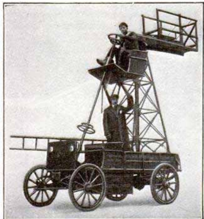
One Man Cleaned and Inserted New Carbons in 165 Lamps in Six Hours with This "Trimmers' Truck"
