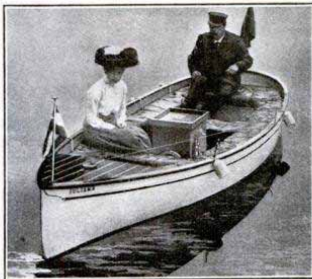
Concrete Motorboat Built in Holland
