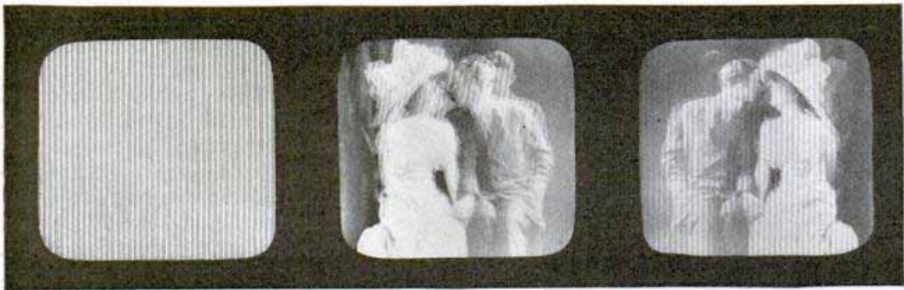
Left—The Screen; Middle—The Magic-Lantern Slide Made from the Three Pictures Seen Above; Right—The Slide with Screen Superposed to Cover Two of the Pictures. The screen is actually much finer than appears in the cuts, which had to be "faked" for reproduction purposes. The general idea, however, is well conveyed by these pictures.
