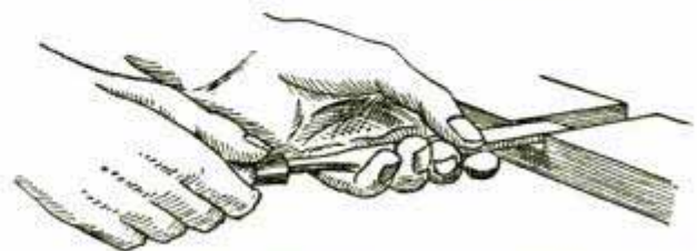
Fig. 72B—Finishing with a Paring Cut
