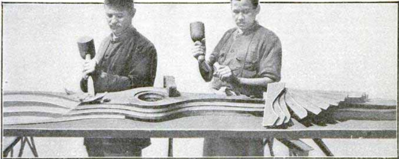
Chiseling the Propeller into Shape from the Rough Glued Sections
