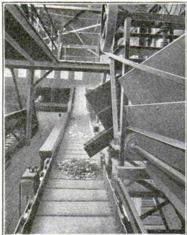
The Coal on This Nut-Picking Table is That Which Fell into the Fourth Screen in the Opposite Illustration. It had to Pass Through a Revolving Screen Before Reaching the Table.
