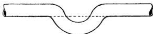
Bend in Pipe
