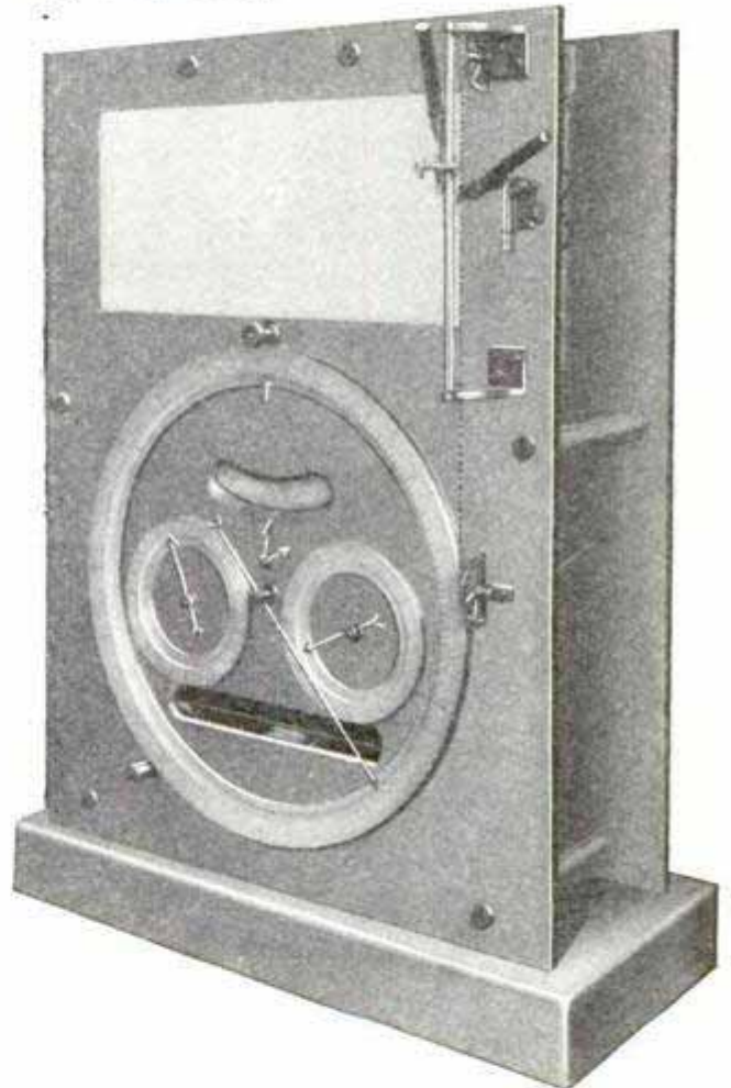
Dials and Curve-Tracing Apparatus at End of Tide-Predicting Machine
