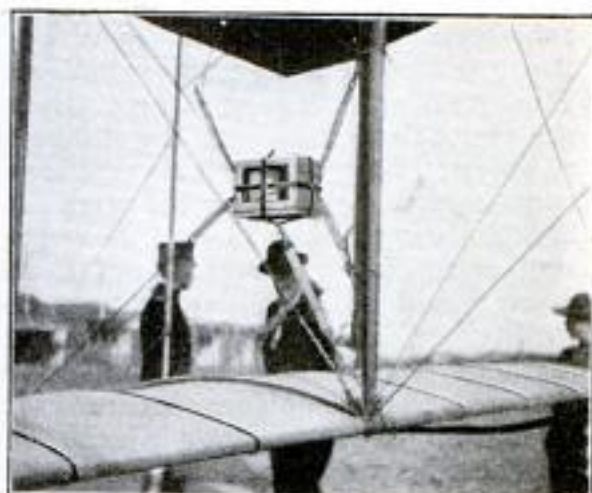
Manner of Securing the Barograph, Used to Measure Altitude, Between Planes of a Biplane.
