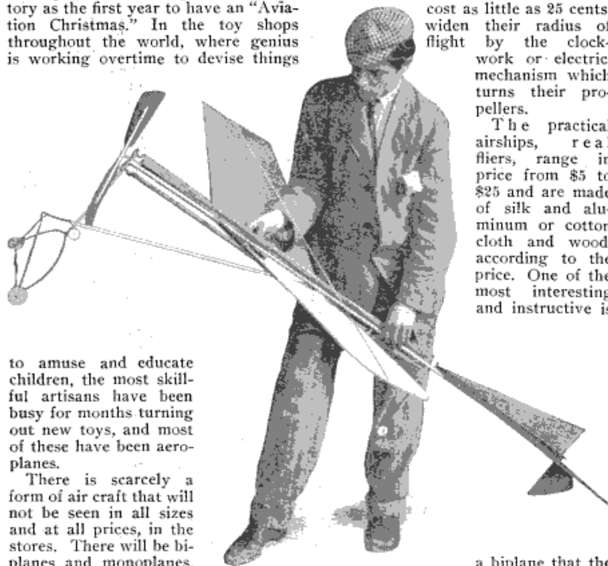
Exact Model of Antoinette Monoplane Made in France, Has Silk Wings and Aluminium Frame—Note the Rubber "Engine" Which Furnishes Power
