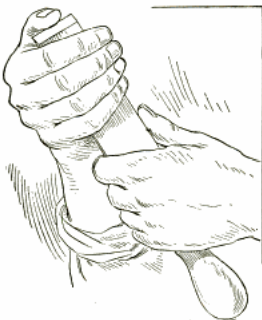
Fig. 52—Testing for Wire Edge
