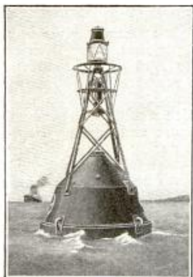
Goodyear Automatic Acetylene and Whistling Buoy—Will Burn a Year Without Attention
