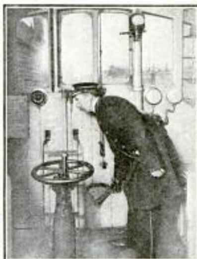
The Guard First of all Pulls over Lever Which Closes Vacuum Break Valve and Sets Pneumatic Slip Apparatus.
