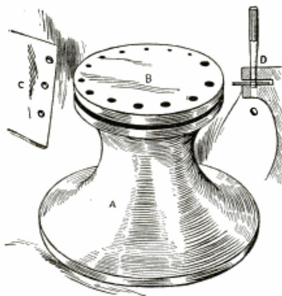
Punching Holes in Sheet Metal
