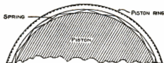
Bent Steel Under the Piston Ring
