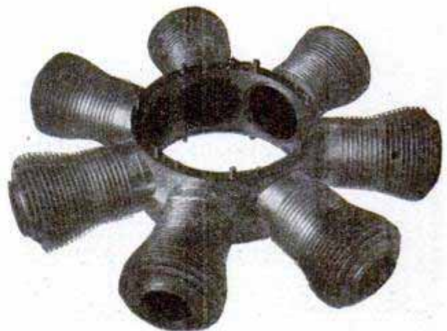
Cylinders Are Cast in One Piece
