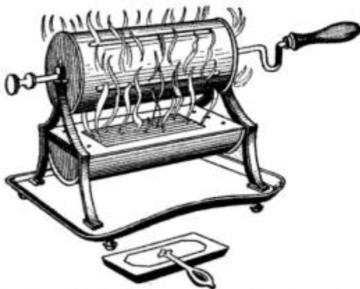
Fig. 20—Alcohol Burner for Roasting Coffee
