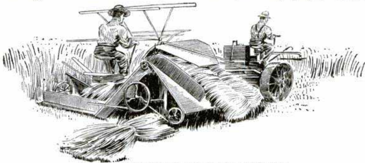
Fig. 24—Alcohol Motor Used in Reaping and Binding
