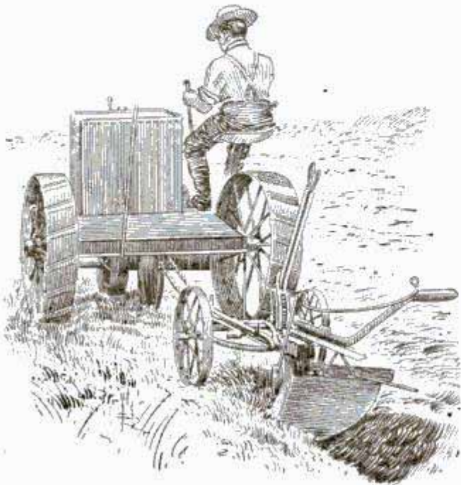
Fig. 22—Adaptation of Alcohol Motor for Plowing
