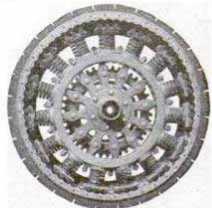
Action of the Springs Under Weight of Car
