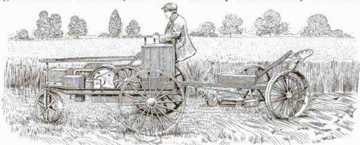
Fig. 23—A Mowing Machine Propelled by an Alcohol Motor
