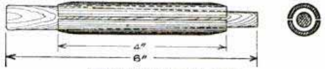
Wood Wedge in the Pipe
