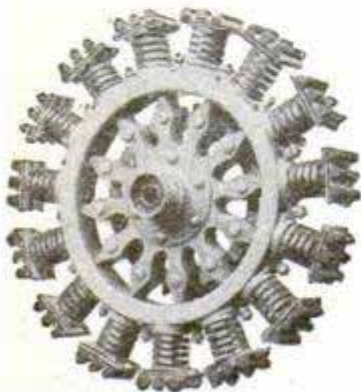
Wheel-Center with Springs in Place
