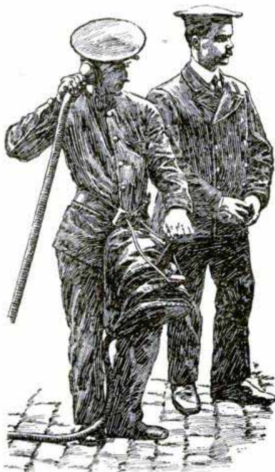
Pumping Air to a Fireman
