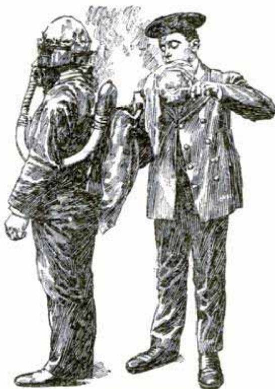
Filling Life Helmet with Liquid Air
