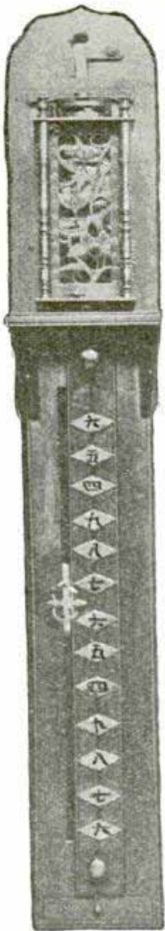
Fig. 16—Japanese Clock with Vertical Dial, Weight and Balance.
