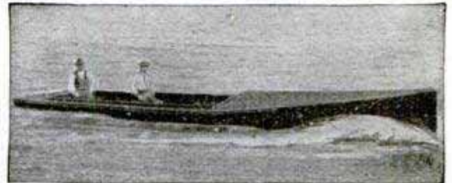
SPEED —C. H. Hunt, of Paducah, Ky., making 15 miles an hour in his 2-cylinder, 12 H. P. gasoline motor boat "Magnolia."
