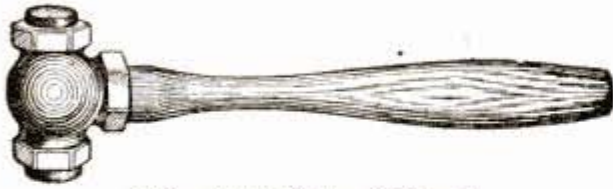
Valve Part Filled with Lead
