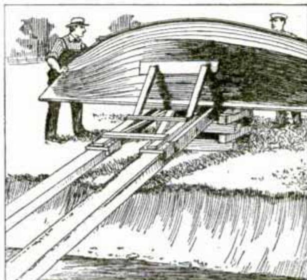
Launching a Boat Sideways
