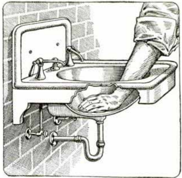
Pushing Out the Obstruction
