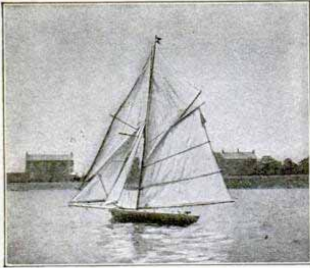
The foresail is held out at an angle to catch the wind and pull head of boat over onto port tack; then foresail is released and all sails and helm take their proper positions and another tack is commenced.
