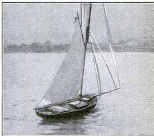
1—Nicely under sail. 2—End of starboard tack; helm is put down; forward sails are slacked away in order to bring her head up into the wind, or "luff." 3—End of port tack; helm is put down and forward sails are slacked away to change tack.
