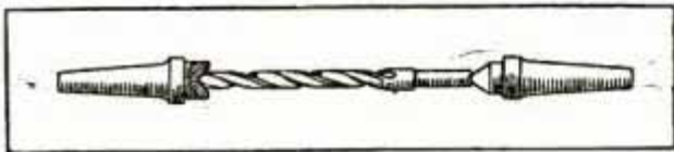
The Cutting Edges Will Turn the Drill
