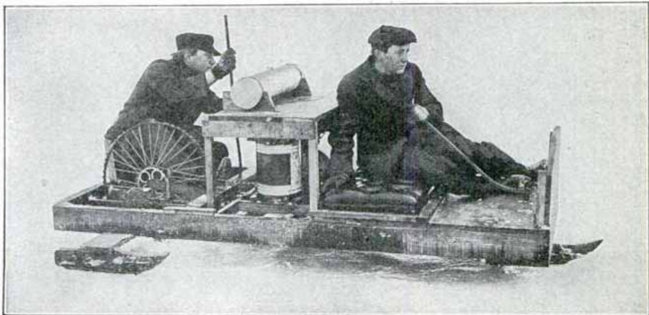
Speed of the Boat Is Controlled by the Upright Lever
