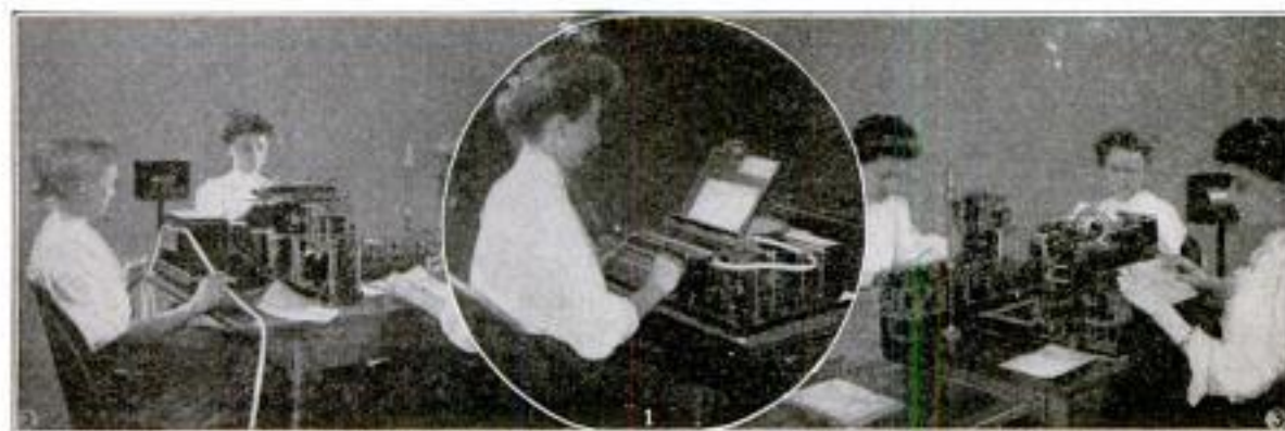
1.—Punching a Message. 2.—Message Going Through Transmitter. 3.—The Receiving Instrument
