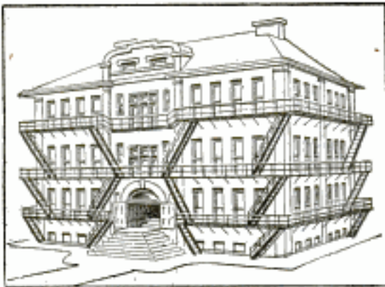
Fire Escape Ladders and Platforms for Each Floor, on Four Sides of Building
