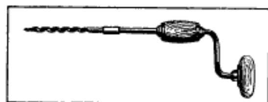
Brace for Boring Pole Tops
