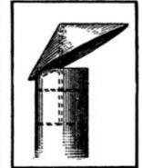
other, for the purpose of fastening a vertical rod, extending about 6 in. above the top of the pipe and terminating in an eye at the top. A conical cap is then made of sheet iron and fastened to the end of the rod by means of a second eye, which passes through the eye at the end of the rod. This allows the wind to tilt the cap in any direction, thus
