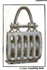
Four of them have been finished lately for Carnegie the Steel Co., and the cut gives an idea what big fellows they are. The height over all of each block is 4 ft. 5 in., and the weight is The 640 lb. sheave pin is of
