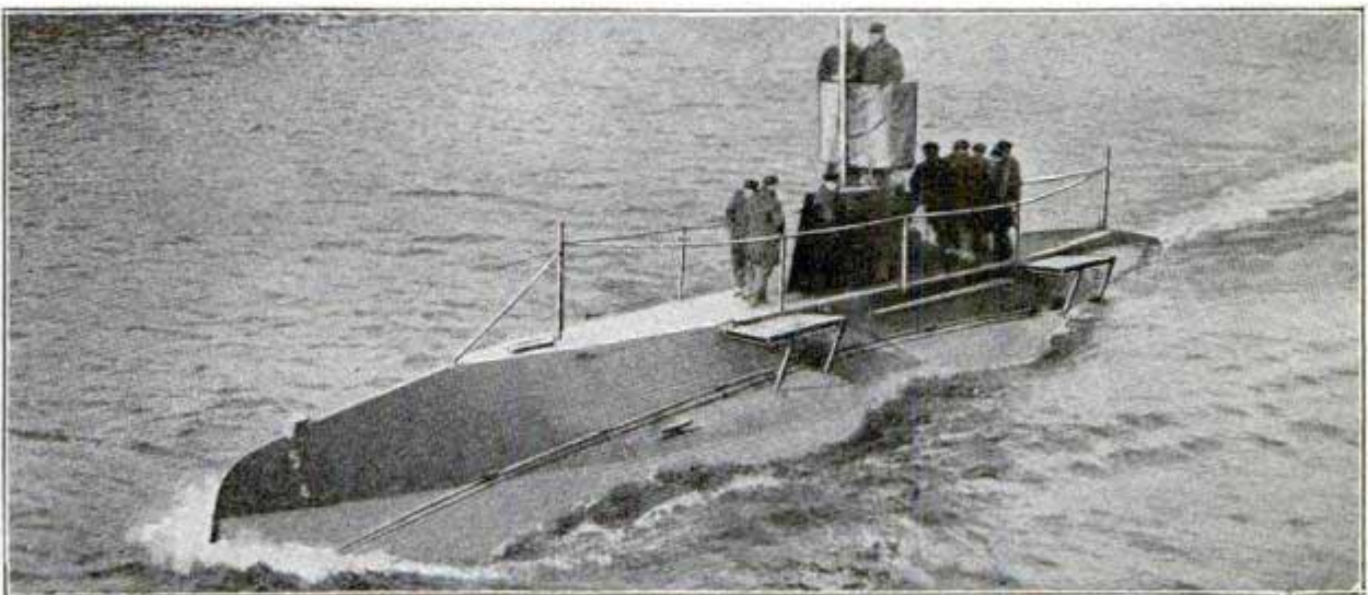
NEW SUBMARINE "OCTOPUS" the Largest in the U. S. Navy, on Trial Test—What Appear to be Platforms Are Hydroplanes to Prevent "Plunging."
