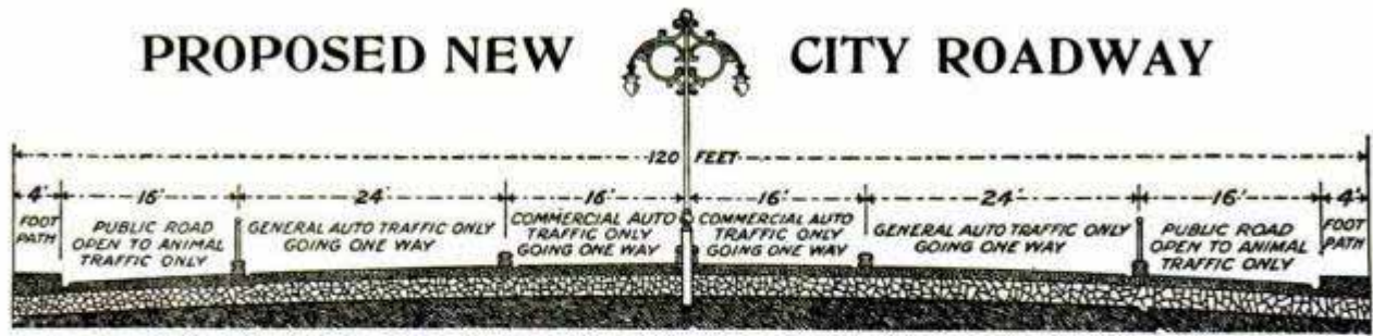
Cross Section of Commercial Roadway
