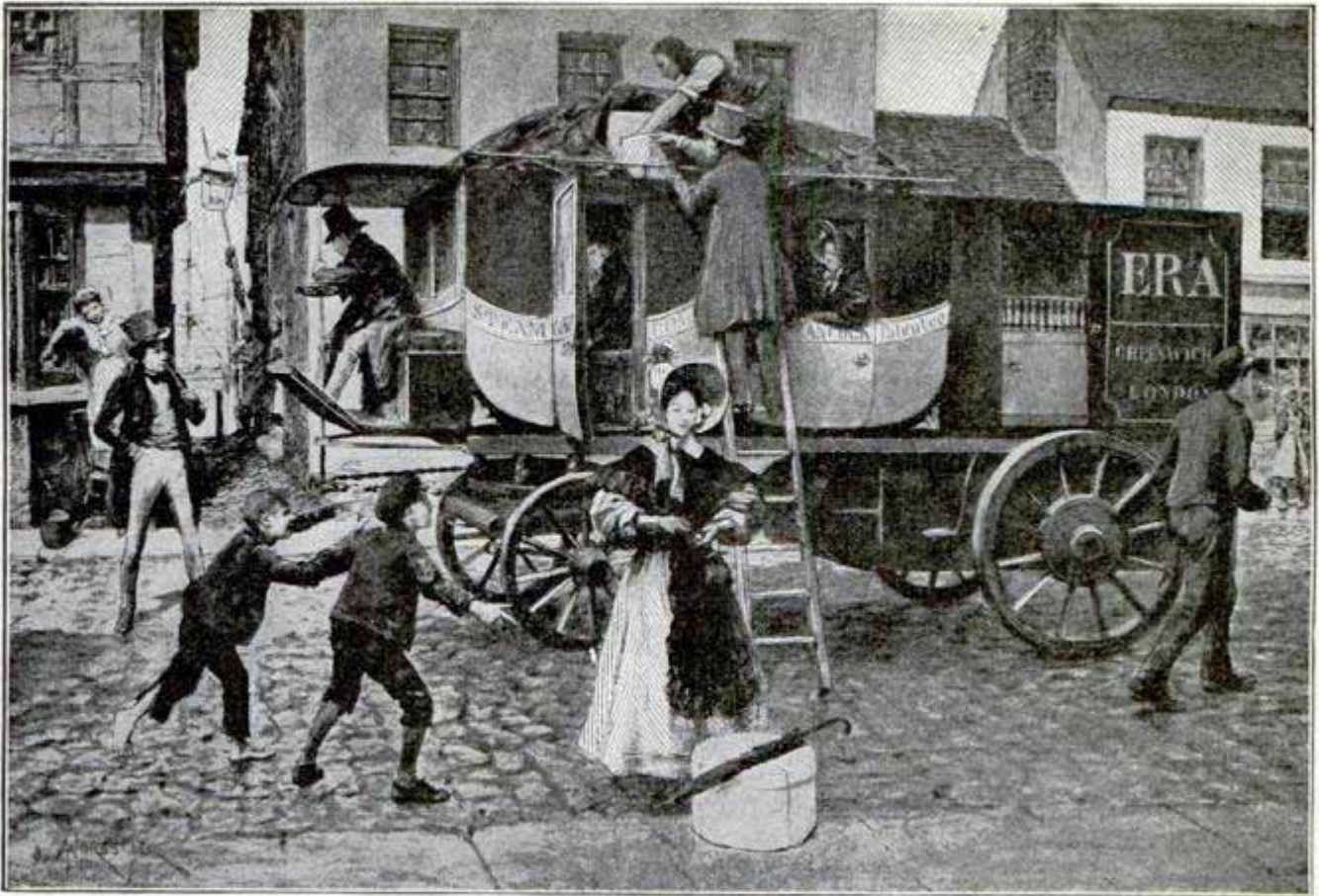
AN EARLY AUTOMOBILE. —Hancock's steam-coach, the "Era," plied the roads daily between London and Greenwich in 1833, just 73 years ago. The ponderous vehicle resembled two stage-coaches on end, with a rear compartment like a mail or luggage van. Parcels were carried on top also. The inventor claimed that he could keep up a speed of 10 miles per hour with his machine, but the record does not state that he demonstrated the matter.
