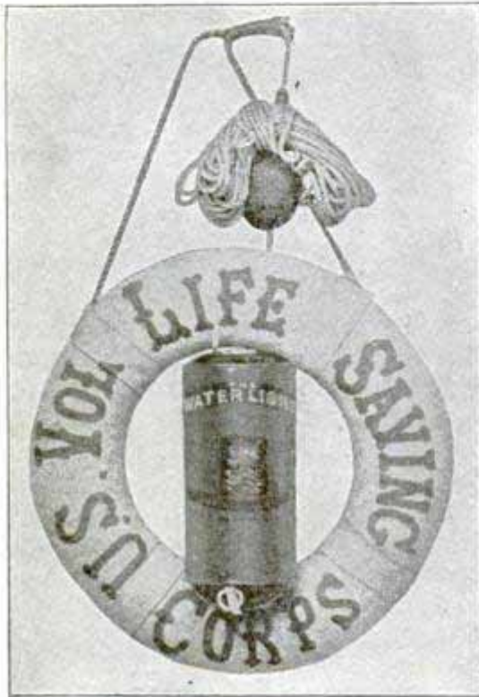
Light Attached to a Life Buoy
