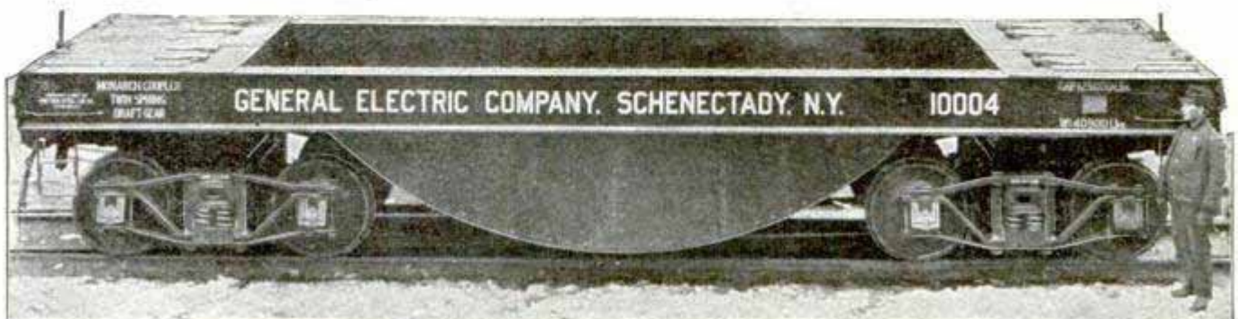
Flat Cars for Transporting Parts of Electric Generators
