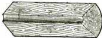
Stave Bolt Ready for Cylinder Saw
