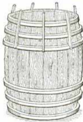
Driving Truss Hoops
