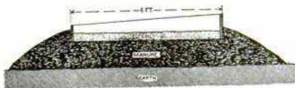
Fig. 2--End View, Temporary Bed
