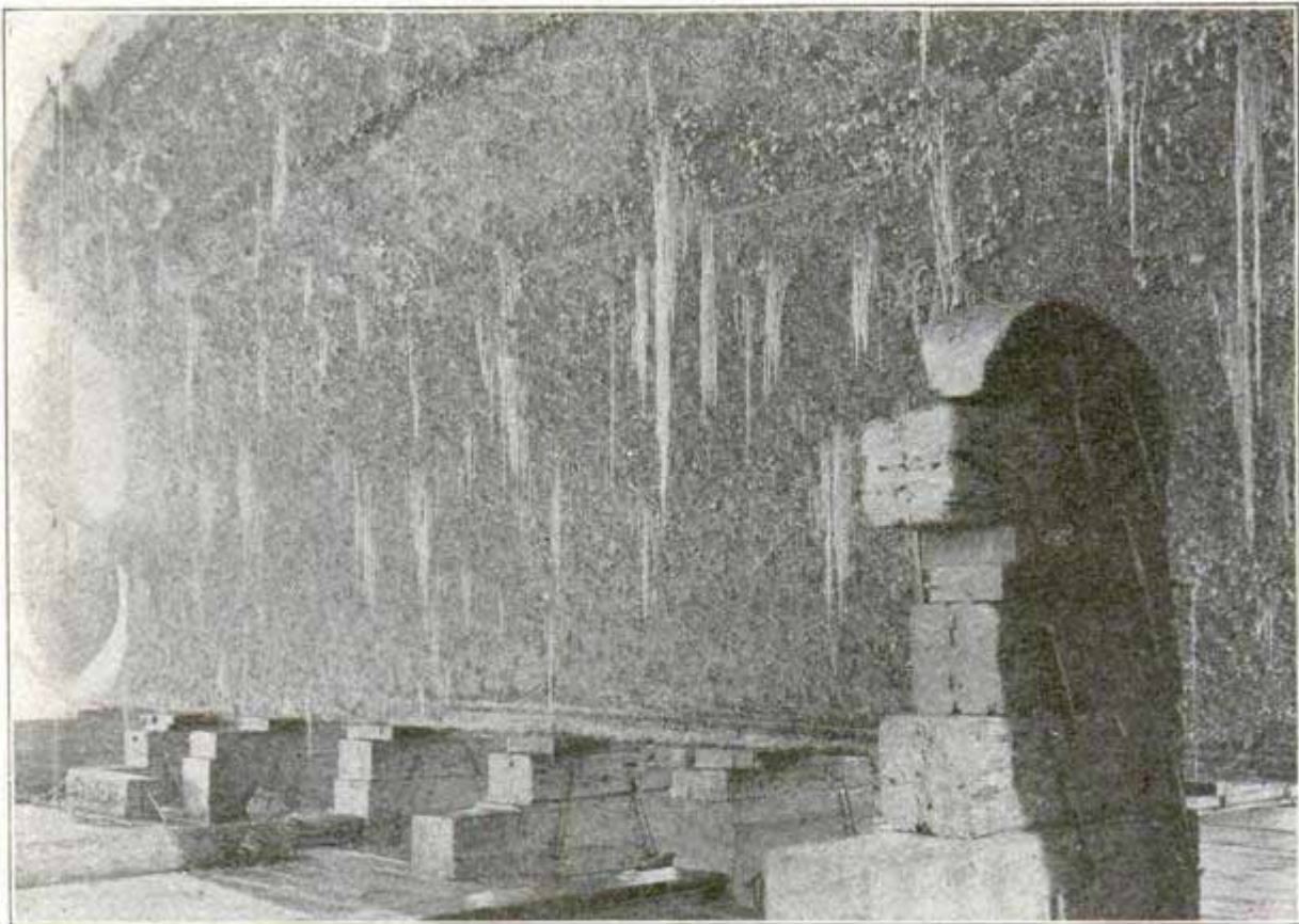
Fig. 5--Hull of Steel Vessel After Cruise of Less than Five Months in Tropical Waters
