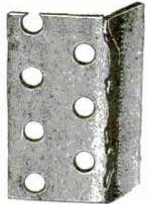
FIG. 3.—A PLATE ALMOST PERFORATED BY A LAP-JOINT CRACK.
