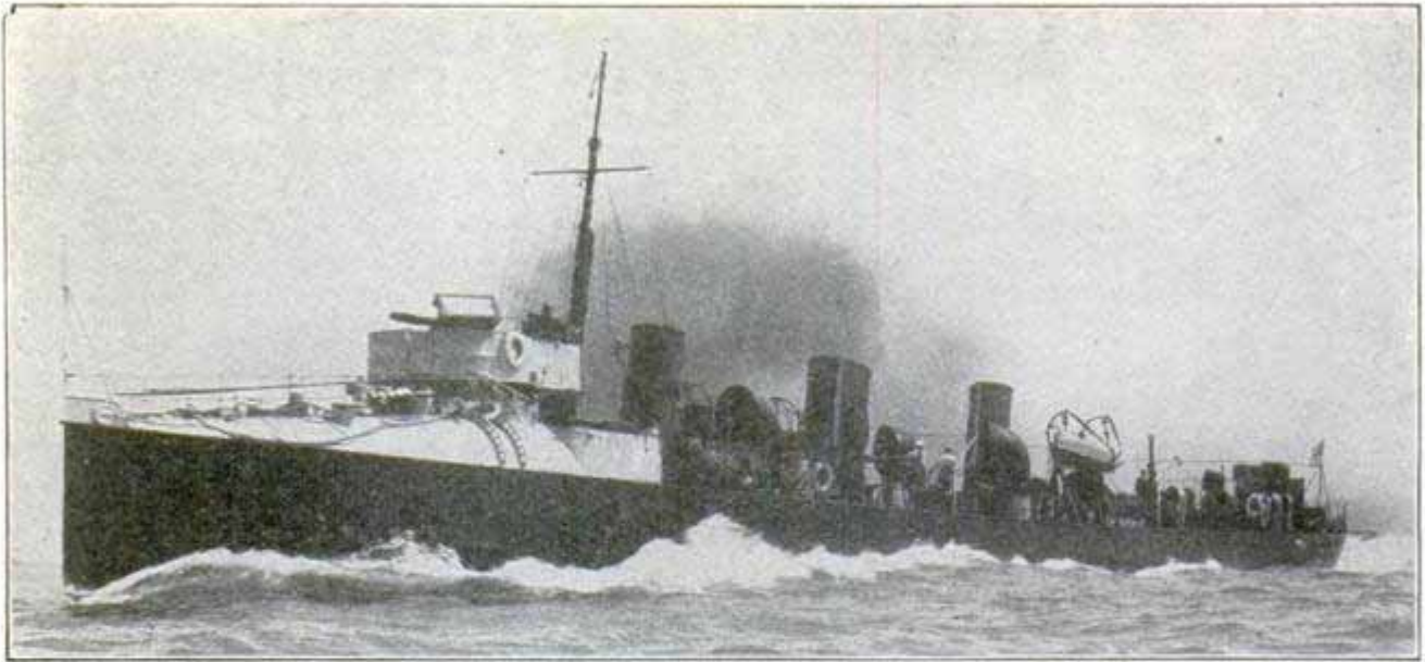
Torpedo-Boat Destroyer "Whiting," Traveling at Over 35 Miles an Hour, and Just About to Discharge Her Bow Torpedo at a Floating Target
