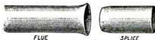
Tipping Boiler Flues
