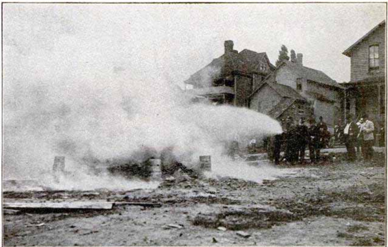
Firemen Extinguishing the Fire at a Distance of 20 Feet During Rapid Discharge of Cartridges
