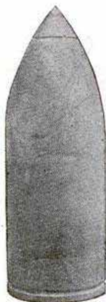
Armour-Piercing Shot (6-in.) After Penetrating Plate
