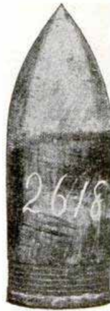
Penetrated 9-in. Plate Twice and was not Injured
