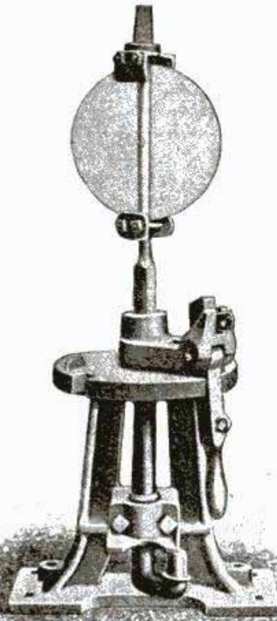
STANDARD MAIN LINE LOW STAND SWITCH STAND: To change the switch it is necessary to raise the handle or lever from its present vertical position to a horizontal position before it can be moved to the left, which action shifts the switch-points. The lever is then pushed down until it occupies the notch shown, when the lever can be locked with a padlock, and the switch-points held firmly.
