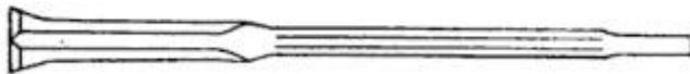
Type of drill used in Rocky mountain mining districts. Cross-formed bar welded onto octagon bar; shank forged to small bushing.
