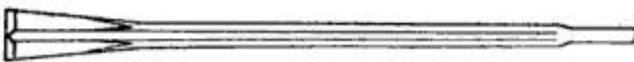
Type of drill used in Michigan copper and iron mines. Long cross upset in bolt upsetting machine from octagon bar.
