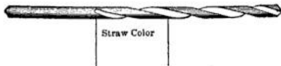
To Keep Small Drills From Breaking
