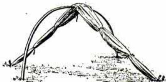
Tent upon frame ready to pull in direction desired
