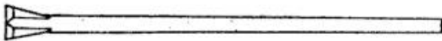
Type of drill as made with a Power Drill Sharpener. Cross upset 3 inches long from round bar; no forging down of shank, as chuck bushing is large enough to take the full size of bar; the most economical drill that can be made.
