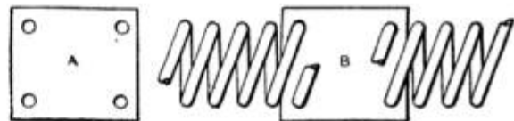
Spiral Spring Repaired
