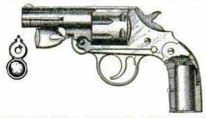
burglars and hold-up men, as an assailant would be blinded and dazed by the sudden flash of the light thrown directly on his face besides offering an easier target than the man whose exact position could only be guessed at. The battery is located in a chamber in the handle of the revolver and is connected with the lamp by a wire running through the stock.
