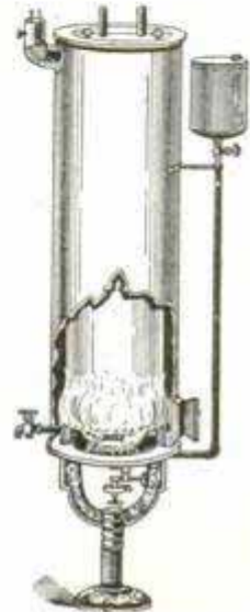
Fig. 2.—Burner Using Gasoline as a Fuel.
