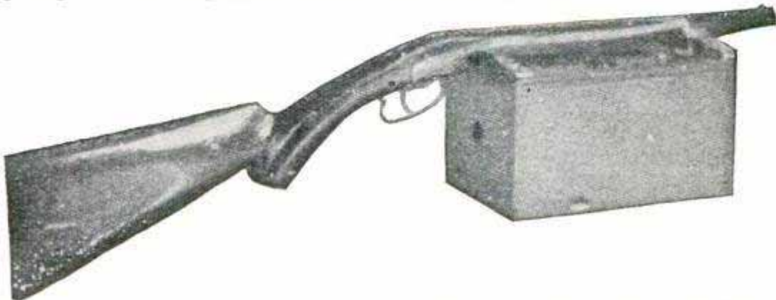
Gun Camera for Photographing Moving Birds and Fish
