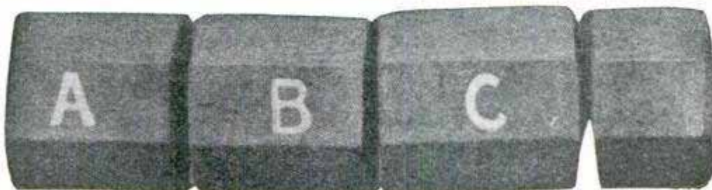
Fig. 1.—Steel Ingot for Three Wheels
