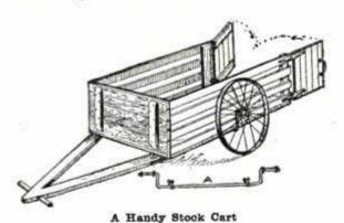
and 5 ft. in length, and bolted to the axle near the middle of the bed. Bolt a cart handle on the front and fit the rear with two doors and a strong latch. Mount the whole on wheels and, according to a correspondent of the Ohio Farmer, you will have a "stock chariot" which cannot be surpassed.
