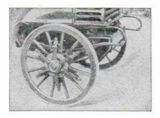
**Hub Springs Replacing Rubber** Tires.
