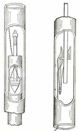
Tools for Fishing Broken Rods and Pipe Out of Wells
