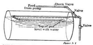
BOILER FEED AND BLOW-OFF ARRANGEMENT.
