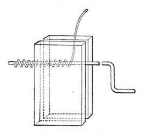
Winding a Coil Spring.
