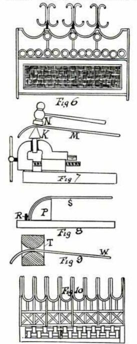
headed up as each addition is made. Thus the series of rings are united and then the side pieces are similarly riveted. The points at the top are then worked out and joined on. These points are filed down to the necessary taper after the union is effected. The finishing work involves smoothing rough places with a file and painting. Asphaltum makes a good black finish. Some of the best designs of grates are bronzed.
