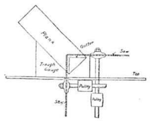
Device for Sawing Wood Gutters
