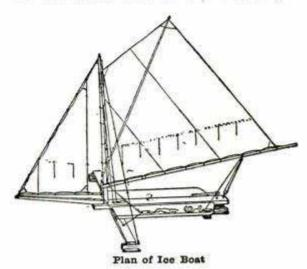
bolt a piece of timber 2x4x22 inches in front of the rudder block, and to this crosspiece and the 6-foot plank nail 8-inch boards to make the platform.
