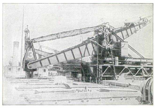
How the Bucket is Lowered into the Hold-Showing the Operation of the Walking-Beam
