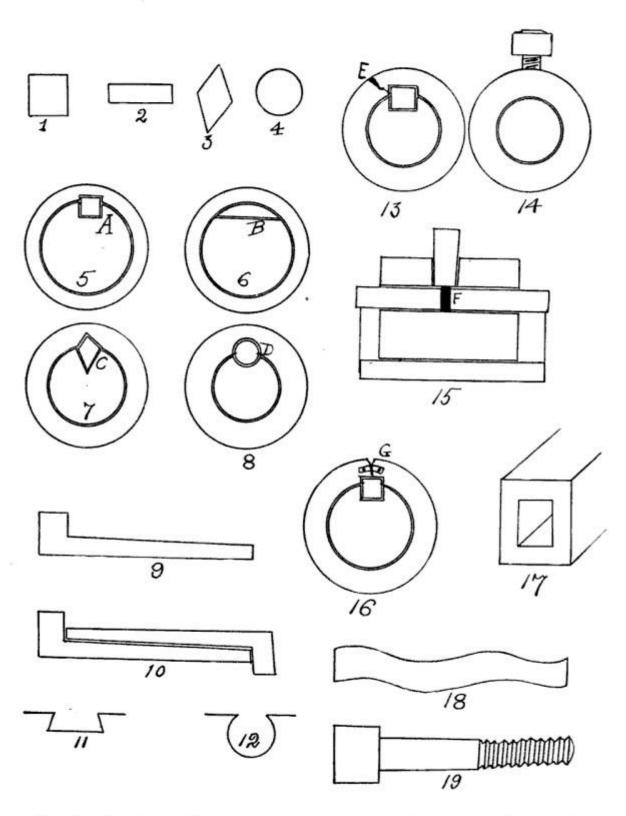
used. The drawing shows the parts at the center bearing where the oil hole is completely closed by the point of the tapering key as at F. This combination ran well for a few weeks, then the stopping of the oil
