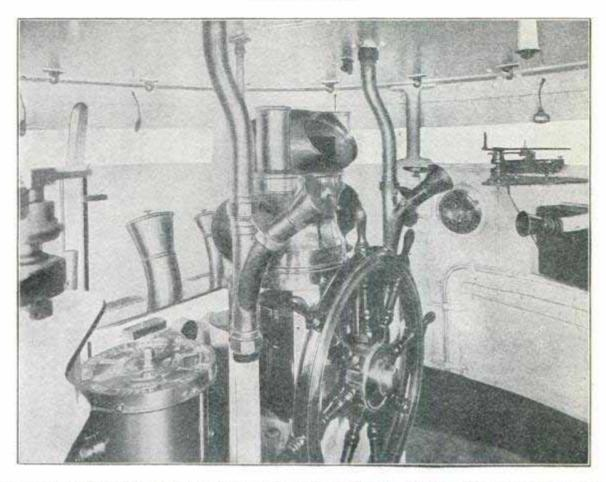
The Conning Tower is the Brain of the Battleship. From this center of intense activity communication leads to every working member of the ship. The engines, rudder, turrets, pumps, guns, torpedoes, signals--all these things are directed from the Conning Tower in time of action. Every part of the ship is made respondent to the touch of a button, the movement of a small lever, or verbal instruction through a perfect system of telephone connection.
