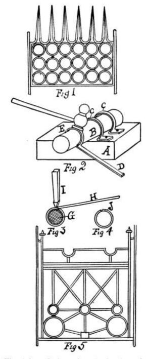
Fig. 1 is a design of grate front used for various purposes in connection with grate fires. The series of rings are united by a rivet between each at the joining point. With thin metal the holes can be punched
