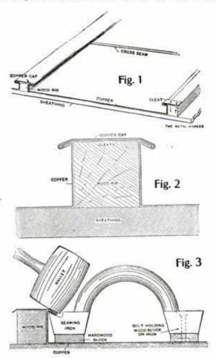
This edge is then cleated at intervals of about 6 or 8 in. to the wood strip. A cap strip of copper, cut about 4 in. wide, is then locked onto the edges of the copper, covering the wood rib and hiding the cleats. No nails should be driven through the copper. The sketch, Fig. 1, shows the method better than any written explanation.
