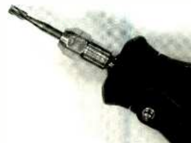
Fig. 3. This is an example of a roto-tool bit useful for cutting slots into copper-clad board. Shown is the Dremel bit #194.
