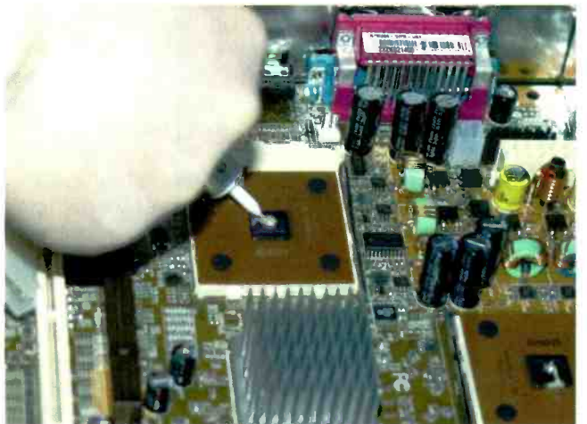
Photo 4. Silver compounds have been found to rival the heat dissipation of plain thermal greases that contain Zinc Oxide or silicone-based grease. Here, some Antec Silver is used to coat the CPU.
