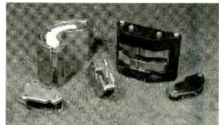
These are the magnet yoke assemblies from several disk drives. The large ones are from older Micropolis (left) and Seagate (right) drives, while the small magnets are from modern diskette drives.
