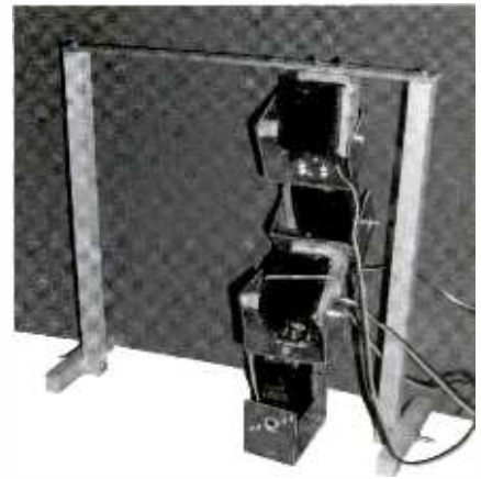
While this stand works, it is a little small (short) for the application. At times the leg can lift and topple itself along with the stand. It appears possible that when both servo motor legs are attached they will be able to lift and walk with the stand in place.
