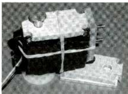
Secure the glued wood components to the servomotor using a couple of rubber bands. Let the glue set for 24 hours before proceeding with the project.
