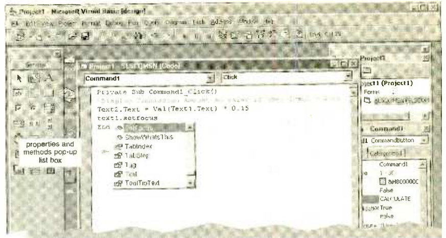
Fig. 2. This screen shot shows a block of code called a subroutine. Coding is made up of many subroutines, and each subroutine is attached to an object. For example this particular subroutine is taking the value of one textbox—or object—and multiplying it by 15%. Visual Basic programming uses dot notation to identify the objects and their properties.
