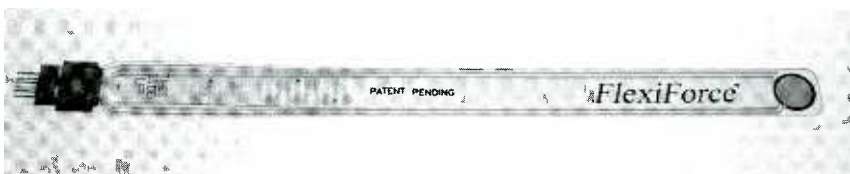
The sensor is a flexi-force pressure sensor. This particular sensor is made to detect pressure from 0 to 1 lb. While the final weight of the robot may be slightly more than the sensor's top weight, I feel it's a better (more sensitive) choice than taking the next sensor that measures pressure between 0 and 25 lbs.
