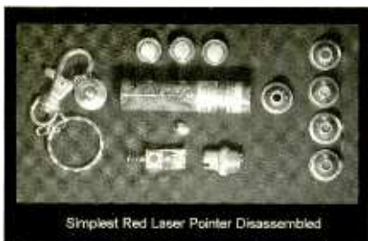
Here's what you get when you crack open one of those bargain laser pointers. As you can see, the parts are minimal—power source, driver, laser.
