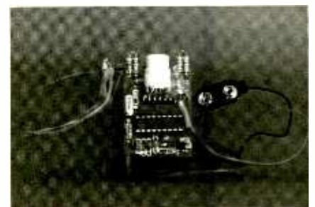
This is the UFO Detector circuit for the vertical model. Notice that the sensor is aligned to the top of the board and the LED is mounted off of the PCB.
