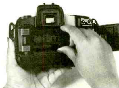
The (e)film cartridge, shown here for the Nikon F5, replaces a 35mm roll of film.
