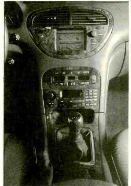
The multi-functional center console on the Peugeot 607 includes a GSM telephone system and a CD-ROM navigation system.
