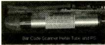
This HeNe laser is the one of the more common types found in supermarket barcode-scanners.
