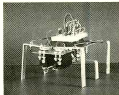
Here is the completed hexapod. A breadboard containing the circuit is mounted to the top of the body. The robot is controlled by a PIC16F84.
