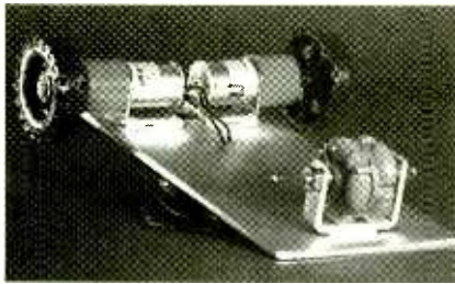
The undercarriage of the vehicle is where the wheels are mounted. Notice the drilled holes for passing the wire through to the top of the vehicle.
