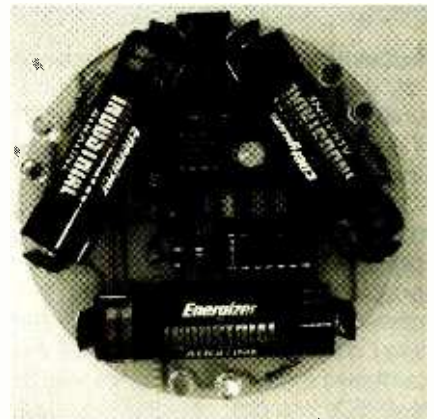
Here is the component side of the circuit. Three batteries form a triangle surrounding the main components. The DC-DC converter is located below the switch at the top of the circuit.
