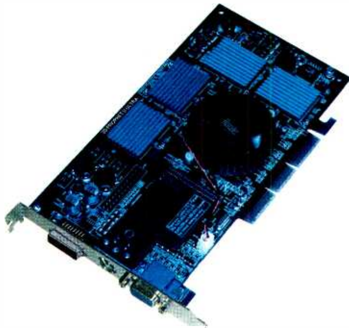
The Hercules 3D Prophet Ultra features a GeForce2 Ultra chipset, 64 MB of DDR RAM, and a processor whose core clock speed equals 259 MHz. Included in the software is 3D Tweak that allows the processor to be overclocked; hence the enormous fan for cooling the board.
