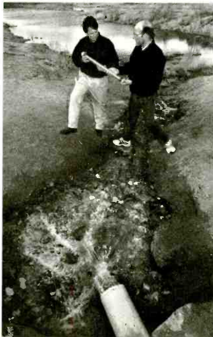
David Teter (l) and Pat Brady are among the Sandia researchers who developed SANS. They are seen here with groundwater flowing through a column of SANS, which would reduce its arsenic content to an undetectable level. (Photo by Randy Montoya.)
