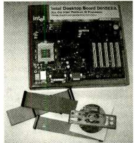
Most motherboards, such as this Intel, come with accessories, including IDE cables and the proper drivers.
