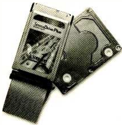
Kingston's StrataDrive Plus comes with a PC-Card interface, letting you transfer the operating system and applications to the new drive without strain or pain.
